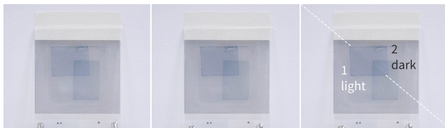
Figure 8: Response of the cyano-chromic interface to dark-light conditions. The top-left rectangle of the EC material changed colour from lighter to darker blue from dark (left) to light (middle) period. The colour comparison (right) of the EC material of the two states.
